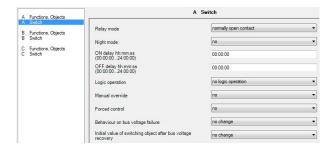
This parameter window is used to set the switching behavior in "Normal mode" of the corresponding actuator output channel..
