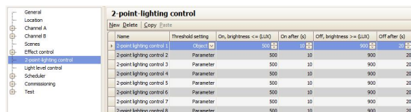
Fig. 28 2-point control parameters window
