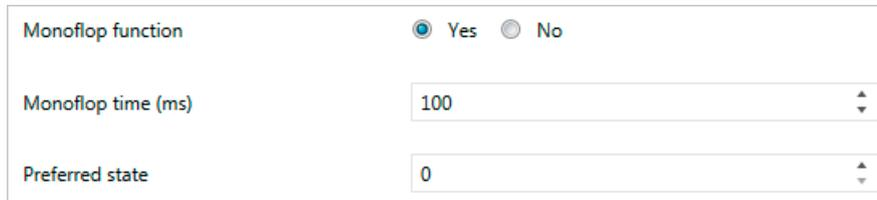
Image 8-20 Data transfer from KNX to LOGO!: Monoflop function
