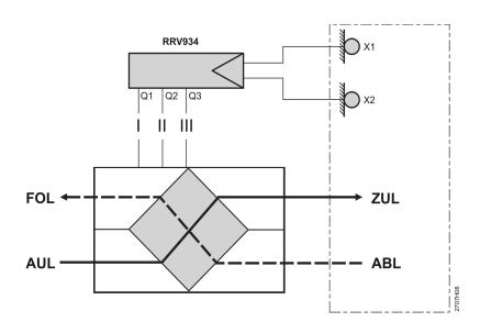
Q1 - Q3 3-stage step selector of ventilation plant X1 Air quality sensor, DC 0...10 V X2 Humidity sensor DC 0...10 V
