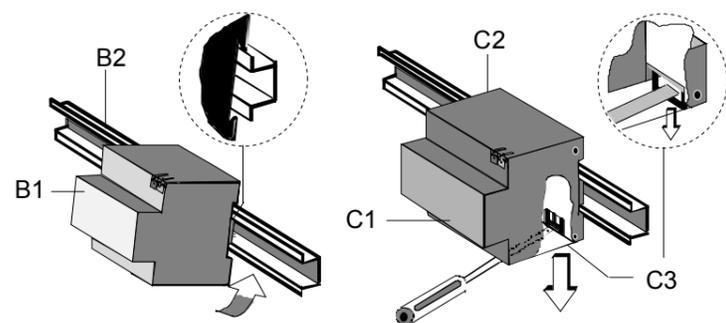
Figure 2: Installing / dismantling the device
