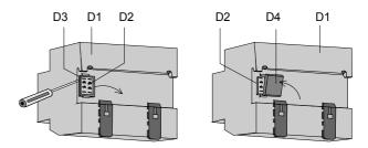
Figure 3: Mounting and dismounting a DIN-rail device
