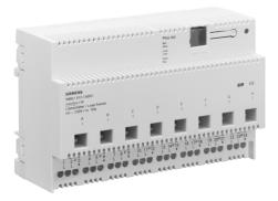
The load switch N 512 is a N-system DIN-rail mounted device. Via its eight outputs it can switch eight separate groups of electric devices. The power supply of the load switch N 512 is provided by the bus (i.e., it requires no additional power supply).
