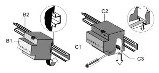
Figure 2: Mounting and dismounting a DIN-rail device
