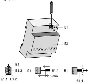
Figure 4: Connecting and disconnecting bus wires
