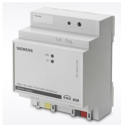
The device serves as an interface between KNX and BACnet. The parameterized KNX communication objects are translated as BACnet objects and can thus communicate into the BACnet world. BACnet clients can either log in via a so-called COV subscription and are automatically informed about KNX events, or they use the Read Property service to query the status of the objects as required.
